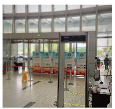
Photo: Automatic temperature measurement of personnel entering the hospital (from the author's own collection, used with permission).
